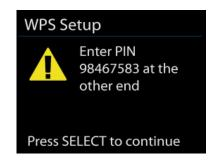
REGENT i450s will generate an 8-digit code that must be entered into the router, access point or other device.
