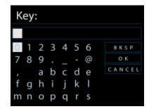
To enter the network key, use the knob or the buttons on the remote control. You can turn the knob to navigate and press to confirm.
