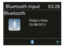
In Bluetooth mode, the REGENT i450s enters pairing mode automatically. You can turn on Bluetooth on your compatible device and search for the REGENT i450s radio to connect. While the REGENT i450s is waiting for pairing, the Bluetooth icon will flash at the bottom of the screen. If the connection is successful, you will hear a short beep and the Bluetooth icon will stop flashing.
