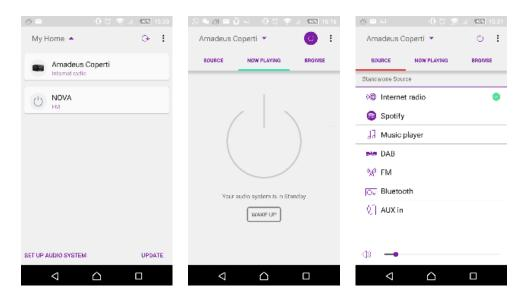
Once your smartphone/tablet has access to the device, it will automatically connect the next time you open the app. Select the desired mode on the home page. You can then control the selected mode on your mobile device and the radio screen simultaneously.
