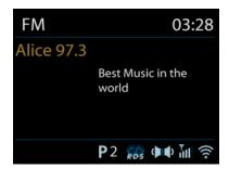
To find a station, press the rotary knob or OK (SCAN) on the remote control. The frequency display begins to light up as the REGENT i450s scans the FM band. Alternatively, you can scan up or down by pressing and holding the buttons, or tune manually by quickly pressing or turning the rotary knob.
