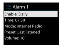
Select Alarms from the main menu to set or change an alarm. Select the alarm number (1 or 2), then configure the following parameters:
