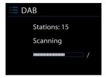
Once the scan is complete, the radio will display a list of available stations. To remove stations that are listed but not available, select "Trim invalid." Turn the navigation knob to display the station list and press to select. Once a station is selected, the screen plays and information about the station, track, or show is displayed.
