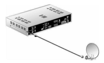
Connect satellite antenna cable directly to the LNB IN socket of the receiver.
