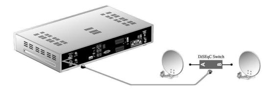
If you want to use a DiSEqC switch for more than one satellite, connect DiSEqC switch OUT to LNB IN connector of the receiver.
