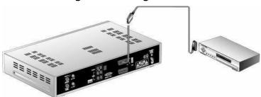
Connect the VCR SCART of Ferguson STB to recording device with fully featured SCART cable.
