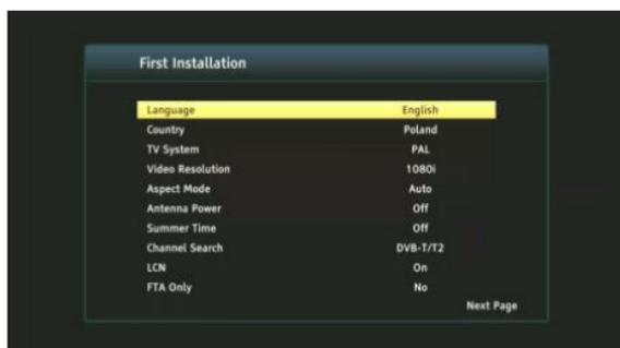
After selecting the settings, go to the "next" item and confirm with the "OK" key. The signal from the antenna will be scanned.
