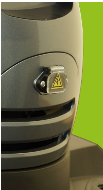
external charging charging the scooter from the outside without removing the battery
