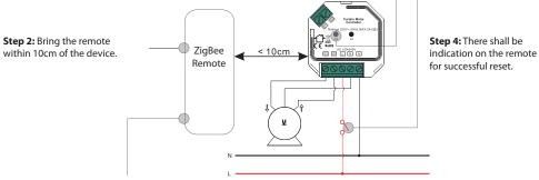
Step 3: Set the remote into Touch Reset procedure to reset the device, please refer to corresponding remote manual to learn how.
