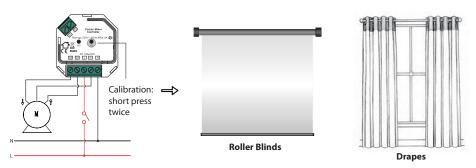
2. Shutter blinds type curtain: short press button K1 four times, calibration starts automatically.
